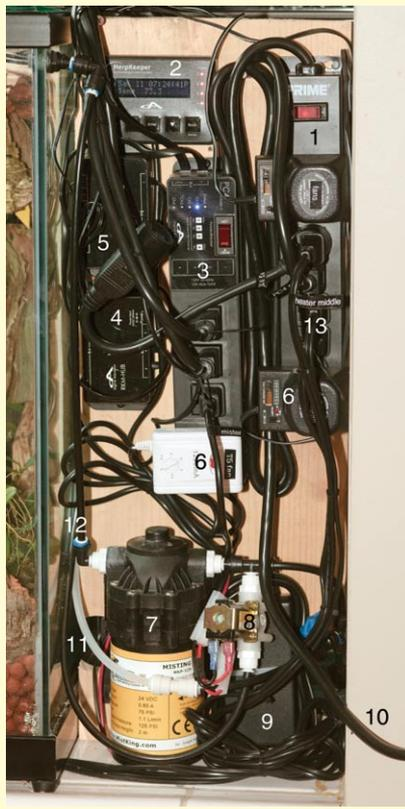
THE automated control for the terrarium's temperature and humidity is based on the Digital Aquatics HerpKeeper system and is mounted on a wood board with all components and wires labeled.
