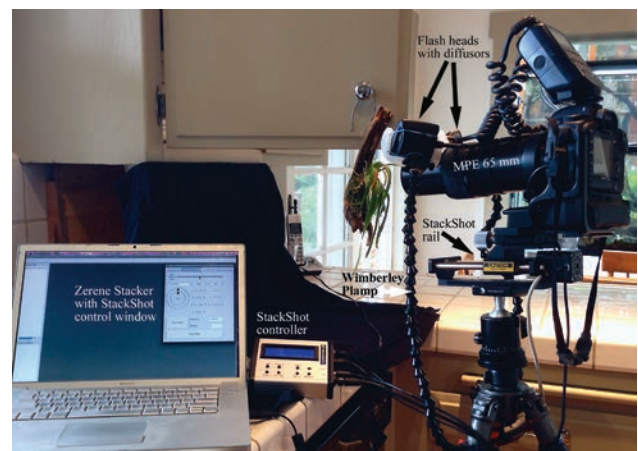
The Cognysis StackShot set-up in the author's “studio,” aka the kitchen counter. The image capture is controlled from the laptop computer through Zerene Stacker with StackShot window.
