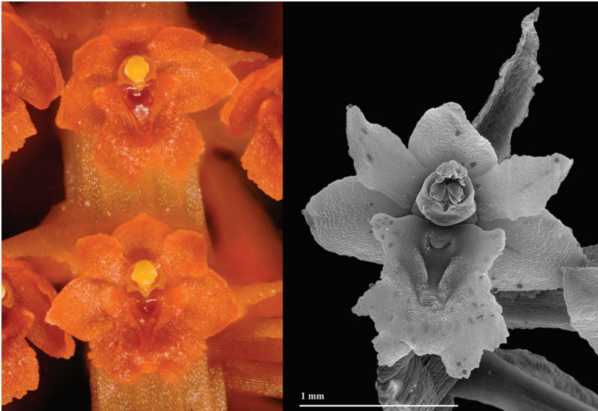
Comparison of z-stacked light micrograph (19 frames) and single scanning electron microscopy image of an orchid flower. Notice the greater detail of the SEM, while color can only be recorded by images recorded with light. Light micrograph on Zeiss SteREO Discovery.V12 with 0.63x plan apochromatic lens, Zeiss Axiocam HRc, processed with Helicon Focus.
