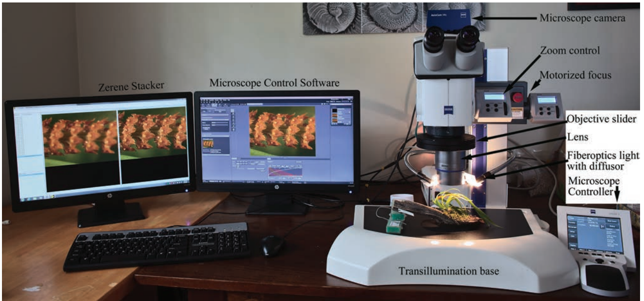
Stereomicroscope Zeiss Discovery.V20 with blue Carl Zeiss AxioCam HRc microscope camera (peltier cooled CCD). Notice that the lens is off-center to ensure that the optical axis is parallel with the z-axis.
